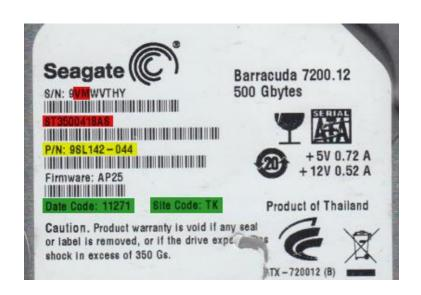
These drives can be identified by **NOT** containing a period (.) in the firmware number. Use the following criteria to find a donor drive.
